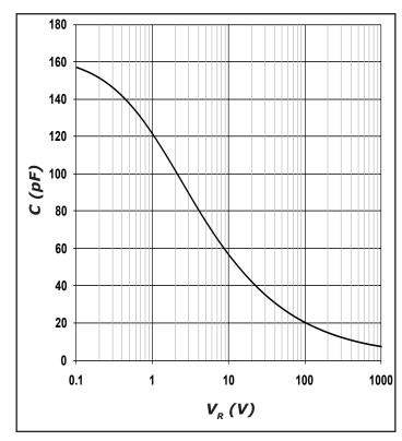
Figure 6. Capacitance vs. Reverse Voltage
