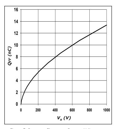
Figure 5. Recovery Charge vs. Reverse Voltage
