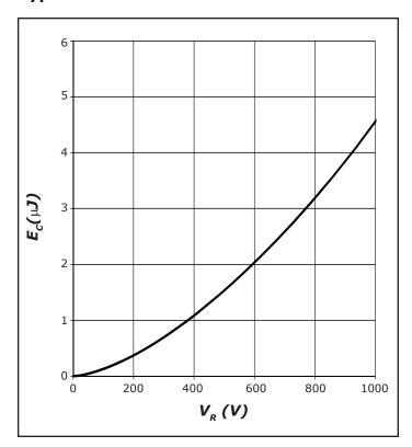
Figure 7. Typical Capacitance Stored Energy
