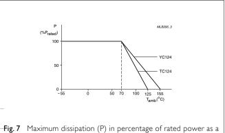
fig. 7 Maximum dissipation (F) in percentage of rated power as a function of the operating ambient temperature  $(T_{amb})$
