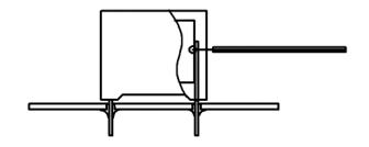
Temperature monitored inside the capacitor.
