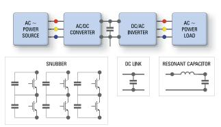
KC-LINK COG dielectric technology also exhibits high mechanical robustness compared to other dielectric technologies, allowing the capacitor to be mounted without the use of lead frames. This provides extremely low effective series inductance (ESL) increasing the operating frequency range allowing for further miniaturization.
