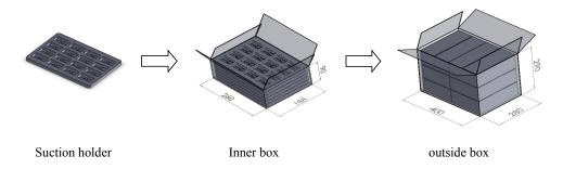
Packaging of snap-in and lead types supercapacitor:
