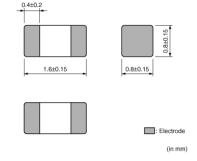
The chip ferrite beads BLM series is designed to work nearly as a resistor at noise frequencies, which greatly reduces the possibility of resonance and leaves signal wave forms undistorted.
