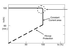
Typical LED power supply I-V curve
