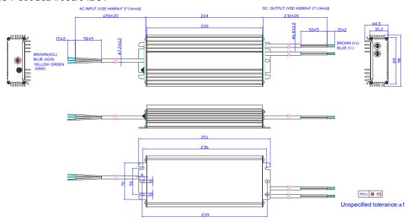
**Note:** The 2 DC output cables are connected in parallel internally because one 1.0mm<sup>2</sup> wire can only carry 10A. Please connect the 2 brown wires together and 2 blue wires together in application, or ensure each cable carries same current.
