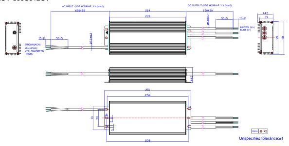
**Note:** The 3 DC output cables are connected in parallel internally because one 1.0mm<sup>2</sup> wire can only carry 10A. Please connect the 3 brown wires together and 3 blue wires together in application, or ensure each cable carries same current.
