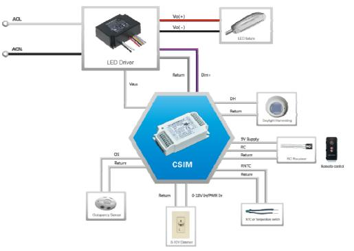
An external auxiliary power supply also can be used to power CSIM and other sensors if LED driver cannot provide auxiliary power.
