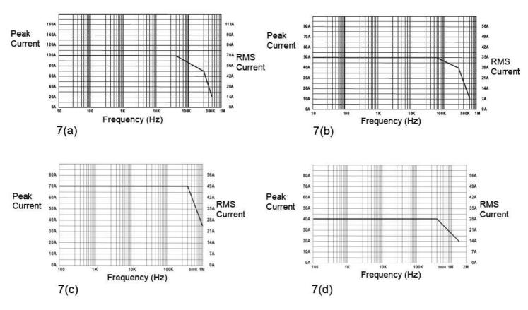
7 (a) – 7 (d) refers to the different models TT-CC 220, TT-CC 550, TT-CC 770, TT-CC 990
