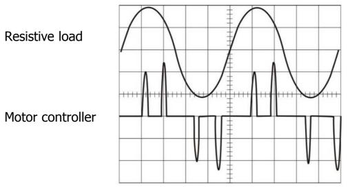
Figure 3: Typical current waveforms
