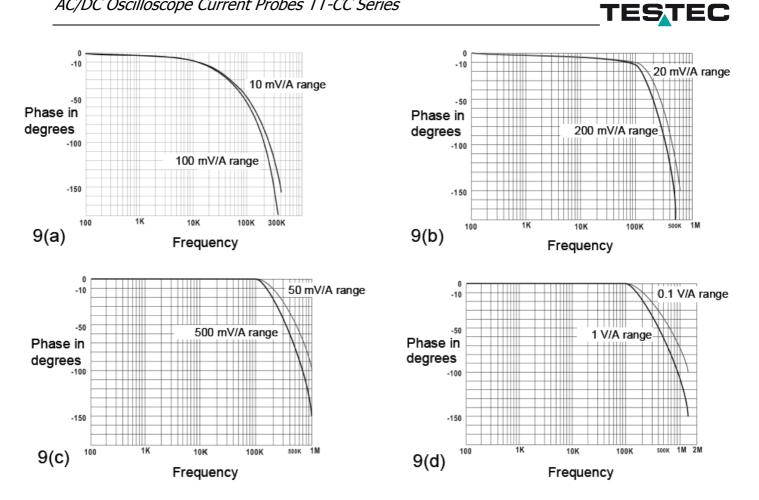
9 (a) – 9 (d) refers to the different models TT-CC 220, TT-CC 550, TT-CC 770, TT-CC 990
