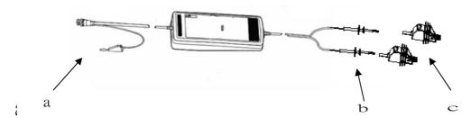
a. Output Cable The BNC output connector and an auxiliary grounding terminal
