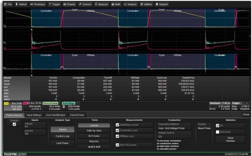
Switching transitions, conduction losses and off-state losses are color-coded and automatically calculated. Measurements are displayed as energy (joules), mean or peak power (watts). For discontinuous supplies, off-state loss provides an excellent tool to fine adjust a current probe's DC offset and improve measurement accuracy.
