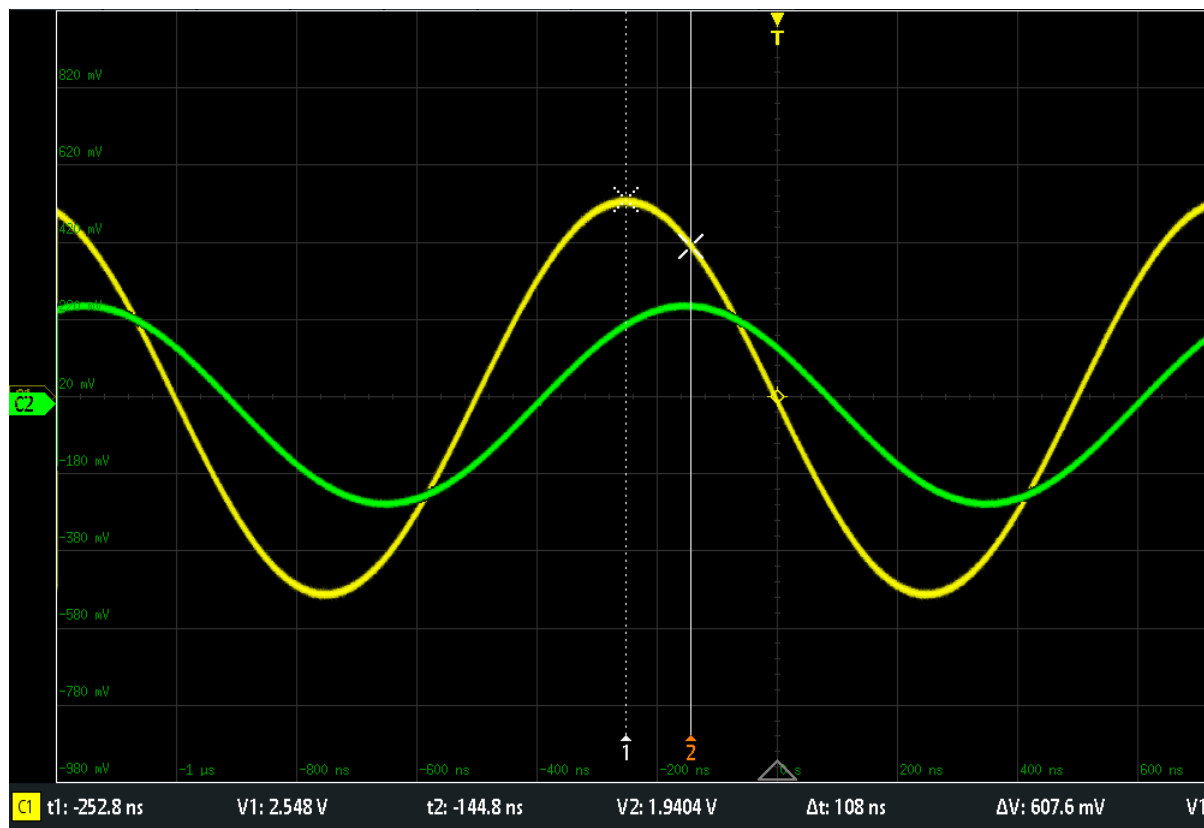
Figure 7-6: Cursor on one source
