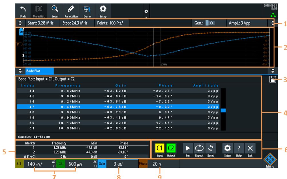
Figure 8-6: Bode plot display
