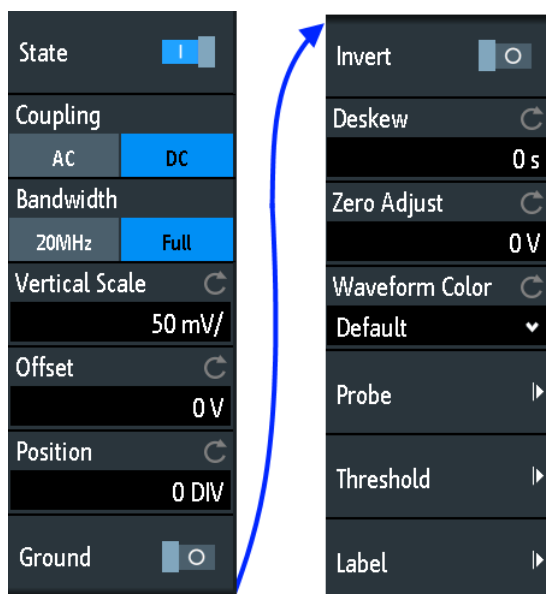
Figure 4-2: Channel menu, split into two halves
