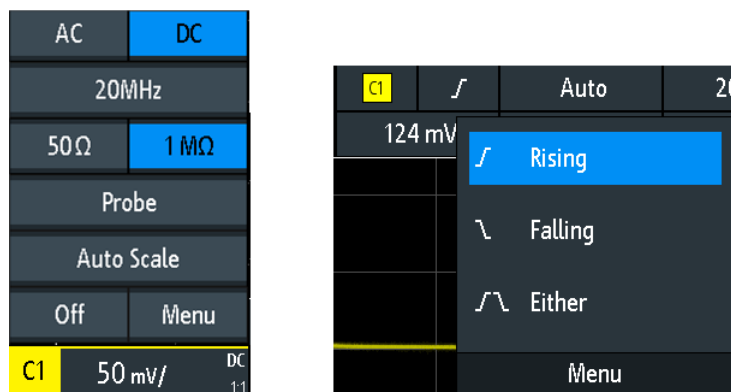
Figure 3-4: Short menus for channel (left) and trigger slope (right)
