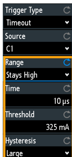
Figure 5-9: Timeout trigger menu
