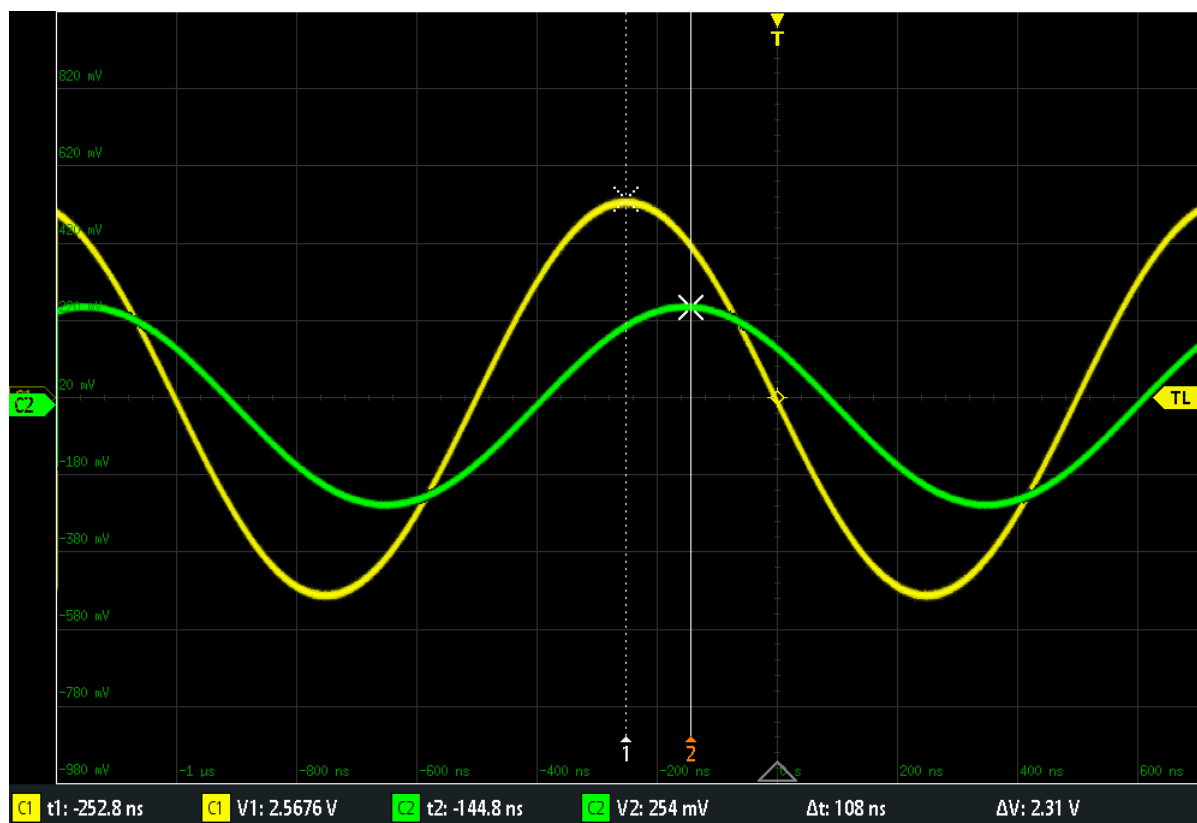
Figure 7-7: Cursor on two sources. Sources are indicated with the measurement results.
