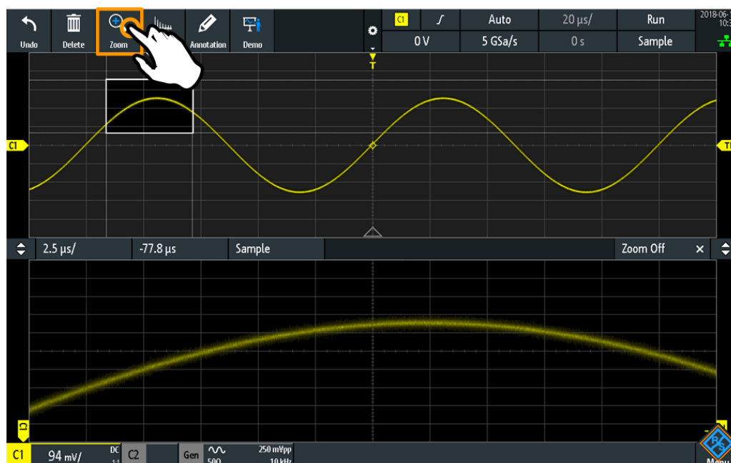
Figure 6-2: Display of vertical zoom
