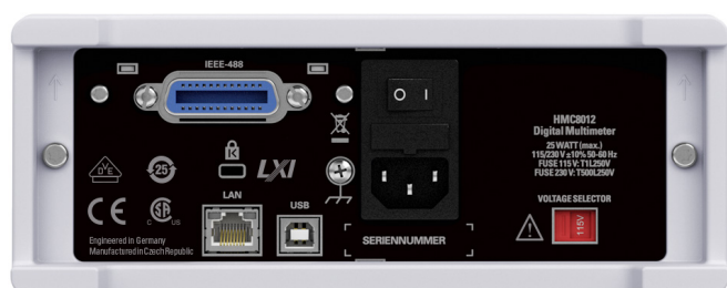
Fig. 1.2: Rear panel of the HMC with voltage selector and connectors
