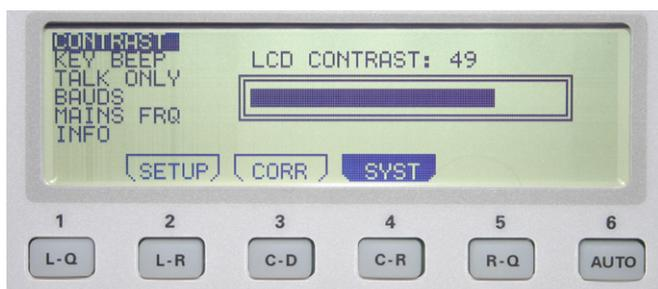
Fig. 5.3: Display of the menu function SYST
