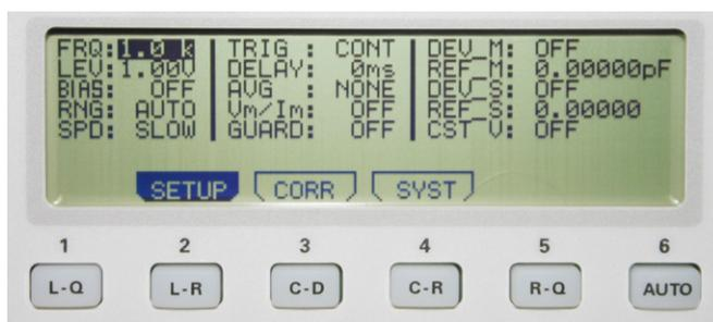
Fig. 5.1: Display of the menu function SETUP
