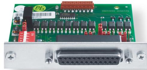
Fig. 7.11: Optional accessory H0118 binning interface.
