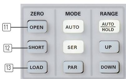
Fig. 6.1: Buttons for the calibration
