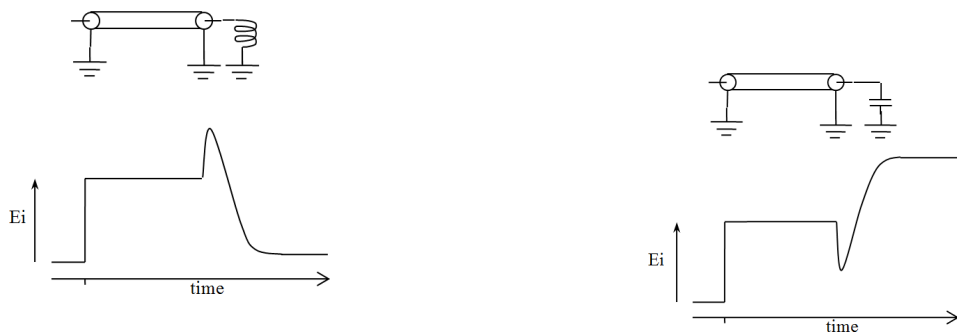
Simplified representation of the response of a reactively terminated line
