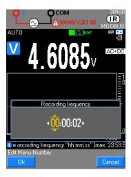
Validating **Freq.** by the [F3] key opens a menu for adjustment of the recording interval in hours, minutes, seconds
