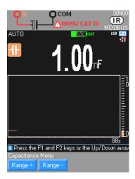
Measurement of the capacitance of a capacitor with a resolution of 1000pts
