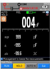
AUTO range selection, automatic (default) or manual: Range + or Range - "Active" protection by PTC thermistor Maximum open-circuit Voltage: 1V typ., 4V max.
