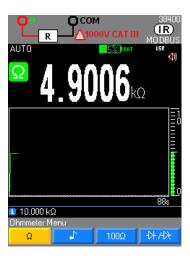
In the 50  $M\Omega$  range, in order to avoid the influence of the mains and guarantee the stated specifications, it is best to disconnect the multimeter from the Wall Plug.
