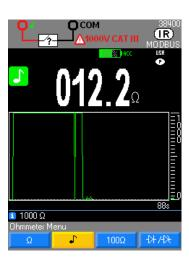
Measurement of a resistance up to  $1000\Omega$  , with continuous 4kHz audible indication.
