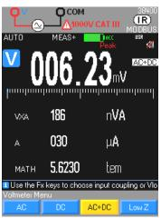
SPEC: directly displays the tolerance of the measurement in progress; there is no need to search for it and calculate it.
