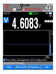
In this stage, it is possible to list the files and to configure the maximum number of records according to the version and the recording frequency or interval (1s is default).
