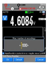
• Programming the number of records Defining a number of records for a measurement campaign makes it possible to stop recording automatically. Selection of the max number of records using the navigator (6500 or 1000 measurements max.); default [F2] is 1000 records
