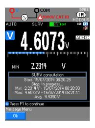
SURV: monitors the variations of a signal, recording the extremes (MIN, MAX) of the main measurement and calculating its mean (AVG).
