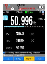
The DCY duty cycle mode is optimized to measure the active or inactive intervals of switching signals or logical signals. Electronic fuel injection systems and switching power supplies, in particular, are controlled by pulses of variable width that can be verified by a duty cycle measurement.
