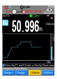
Select the Hz function to measure the frequency of the voltage Measurement of the period is accessible as a secondary measurement If the MLI filter is activated, the frequency that can be measured remains within the pass band limit of the 300Hz filter. Below 10Hz, or if the signal is too weak, the value is forced to "--" Possibility of selection of the range by "Range+ or -" or of the manual freq. F <200kHz (default) or F >200kHz
