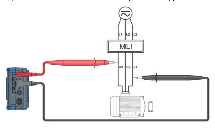
Connecting the multimeter to filter a current >300Hz
