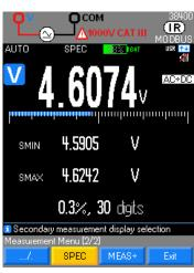
Using the internal technical specifications of the multimeter, the **SPEC** mode directly displays the tolerance on the measurement in progress, with no need to look for it and calculate it.
