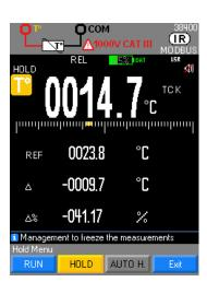
Measurement of the temperature in °Celsius using a thermocouple between the V and COM terminals K thermocouple from -40°C to +1200°C or TCJ (J thermocouple) from -40°C to +750°C
