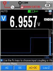
In this setting, the user can measure the true RMS value of an alternating voltage with its bias component (no capacitive coupling): "TRMS" measurement. In the "DC" mode, you measure a direct voltage or the DC component of an AC voltage.
