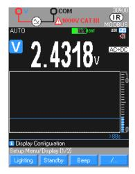
Lighting: selection of 3 levels of back-lighting of the display unit in order to limit the power consumption of the multimeter, as follows: Eco, Normal, Max
