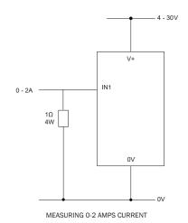
Use a 1  $\Omega$  resistor, with a 4W rating. Setup scaling in software: 0V = 0.00 and 2V = 2.00
