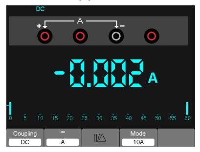
Figure 7-9 DC Current Measurement for 10A
