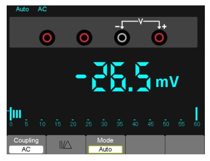
Figure 7-7 AC voltage Measurement
