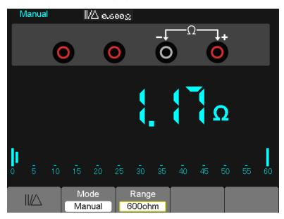
Figure 7-12 Relative Measurement
