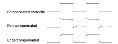
3. If necessary, use a nonmetallic screwdriver to adjust the variable capacity of your probe until the shape of the waveform turns to be the same as the above figure. Repeat this step as necessary. See the figure below for the way of adjustment.
