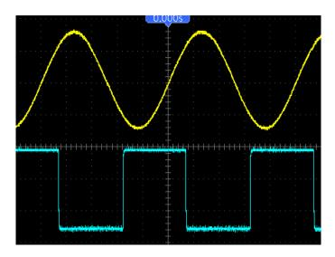
As illustrated in the above figure, input a 1KHz sine wave from CH1 and a 1KHz square wave from CH2.
