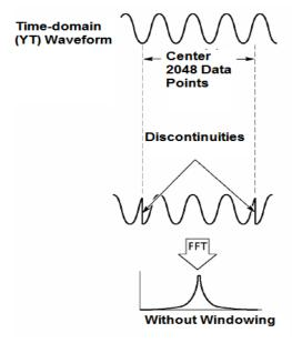
Applying a window to the YT waveform changes the waveform so that the start and stop values are close to each other, which reduces the discontinuities.
