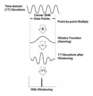
The Math FFT function has three FFT Window options. There is a trade-off between frequency resolution and amplitude accuracy for each type of window. You shall determine which one to choose according to the object you want to measure and the source signal characteristics.
