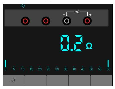
Figure 7-4 On-off Measurement
