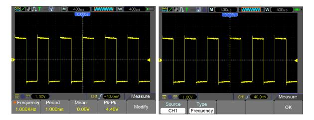
The readouts in big font size on the menu are just results of the corresponding measurements.
