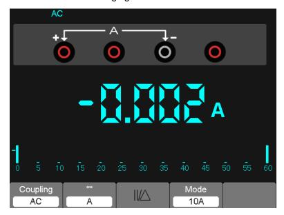
Figure 7-11 AC Current Measurement for 10A
