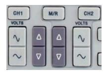
2. **Menu (CH1, CH2):** Display vertical menu options; turn on or off the display of channel waveforms.
