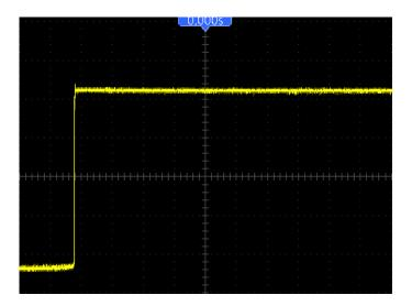
Note: The difference between the overtime and the delay triggers is that the overtime trigger can identify the pulse you need according to your set time and trigger on any point of the pulse. In the other word, the overtime trigger occurs based on pulse identification. It is similar to the > mode of the pulse width trigger, but not the same.
