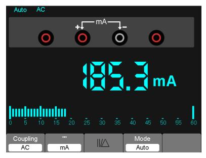
Figure 7-10 AC Current Measurement for 600 mA
