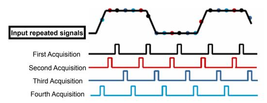
As shown above, acquire input signals (cycle repeatable) for more than once at a slow sample rate,
