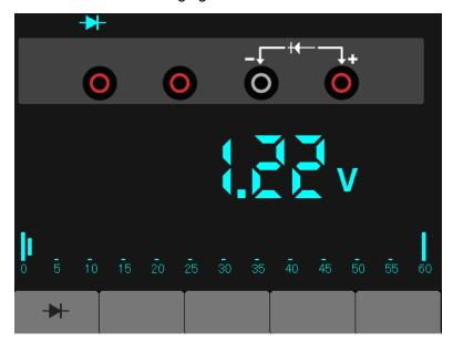
Figure 7-3 Diode Measurement
