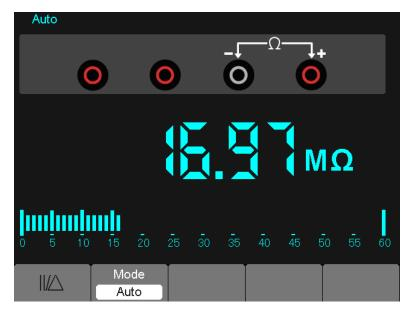
Figure 7-2 Resistance Measurement
