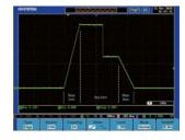
Ramp function of PEL-3000E is able to set the current transition. When turned on. the current takes on a slope form; when turned off, the current takes on a step form.
