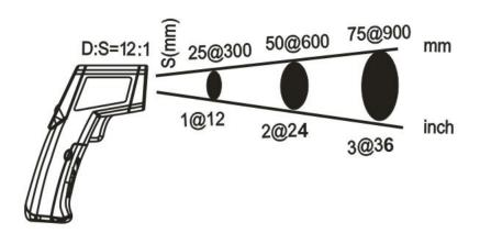
Field of view: Be sure the target area is larger than the unit's spot size. The smaller the target get, the closer the measured distance. For precise measuring, make sure the target is at least twice as large as the spot size. The light-emitting device
