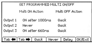
Delay sets a time value in milliseconds between 10ms and 20,000ms (20 seconds)
