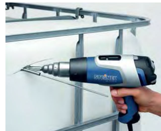
Repairing. Welding PVC water tank.
