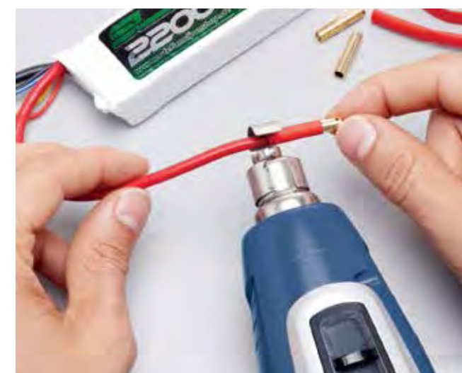
Heat-shrinking. Secure standing for hands-free work.
