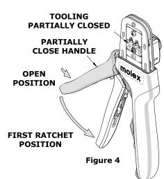
**Note:** The tamper-proof ratchet action will not release the tool until it has been fully closed.
