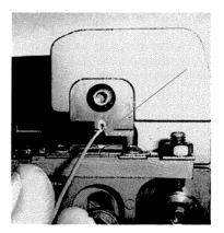
6/ Gently squeeze the handles together whilst ensuring that the wire remains in the correct position relative to the punches.
