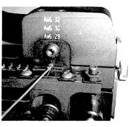
7/ Advance the next contact over the crimping anvils by pushing the yellow feed lever in a right hand direction towards the side of the tool.
