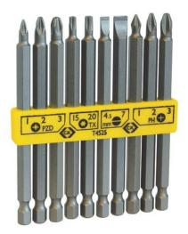
Features & Benefits  $\sim$  Bits made from special S2 Alloy steel  $\sim$  Precision machined tips for an exact screw fit & damage free screwdriving  $\sim$  Length of bits: 100 mm  $\sim$  Contents: Slotted: 4, 5 & 7mm; Pozidriv: 1, 2 & 3; Phillips: 1, 2 & 3; TX: 15 & 20
