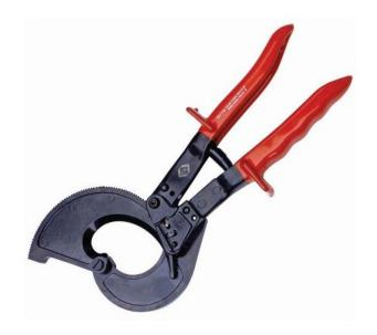
$\sim$  High-grade special tool steel cutting jaws, forged and hardened for an extended working life  $\sim$  Heavy duty ratchet action for the effortless cutting of large diameter cable  $\sim$  Suitable for: Copper and Aluminium cables up to 52 mm Ø SWA cable up to 36 mm Ø  $\sim$  Not designed for ACSR cable or wire rope Features & Benefits
