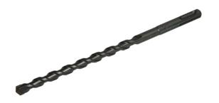
$\sim$  Tungsten carbide tipped with optimized geometry for drilling concrete and stone  $\sim$  Vacuum brazed tips for durability  $\sim$  Ground flutes designed for optimum debris removal  $\sim$  SDS-plus shank  $\sim$  Diameter: 25 mm  $\sim$  Working length: 350 mm  $\sim$  Total length: 450 mm Features & Benefits
