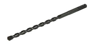
$\sim$  Tungsten carbide tipped with optimized geometry for drilling concrete and stone  $\sim$  Vacuum brazed tips for durability  $\sim$  Ground flutes designed for optimum debris removal  $\sim$  SDS-plus shank  $\sim$  Diameter: 12 mm  $\sim$  Working length: 350 mm  $\sim$  Total length: 450 mm Features & Benefits
