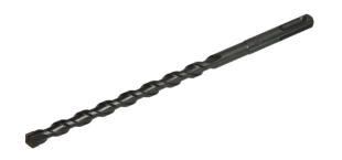
$\sim$  Tungsten carbide tipped with optimized geometry for drilling concrete and stone  $\sim$  Vacuum brazed tips for durability  $\sim$  Ground flutes designed for optimum debris removal  $\sim$  SDS-plus shank  $\sim$  Diameter: 12 mm  $\sim$  Working length: 180 mm  $\sim$  Total length: 260 mm Features & Benefits
