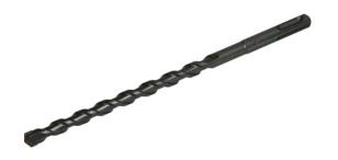
$\sim$  Tungsten carbide tipped with optimized geometry for drilling concrete and stone  $\sim$  Vacuum brazed tips for durability  $\sim$  Ground flutes designed for optimum debris removal  $\sim$  SDS-plus shank  $\sim$  Diameter: 12 mm  $\sim$  Working length: 950 mm  $\sim$  Total length: 1000 mm Features & Benefits
