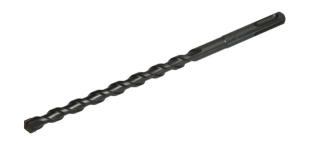
$\sim$  Tungsten carbide tipped with optimized geometry for drilling concrete and stone  $\sim$  Vacuum brazed tips for durability  $\sim$  Ground flutes designed for optimum debris removal  $\sim$  SDS-plus shank  $\sim$  Diameter: 6,5 mm  $\sim$  Working length: 90 mm  $\sim$  Total length: 160 mm Features & Benefits
