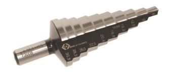
Features & Benefits ~ Centres, drills and deburs sheet metals in one operation ~ HSS, precision ground for accurate drilling ~
