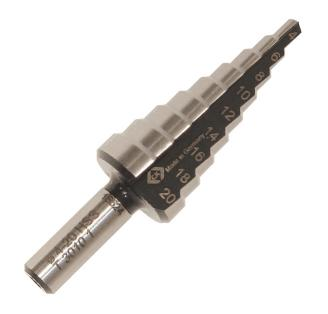
$\sim$  Centres, drills and deburs sheet metals in one operation  $\sim$  HSS, precision ground for accurate drilling  $\sim$  Dual flute construction for faster drilling & longer life  $\sim$  Three flats on drive shaft for secure drive in drill chucks  $\sim$  Cuts hole sizes: 4, 6, 8, 10, 12, 14, 16, 18 & 20mm Features & Benefits
