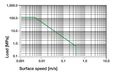
Diagram 01: Permissible pv values for iglidur® A500 bearings with a wall thickness of 1 mm dry running against a steel shaft, at +20 °C, mounted in a steel housing
