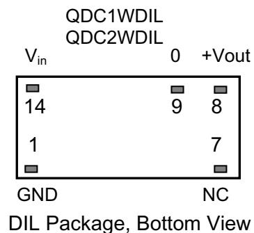
**NOTE:** The NC terminal is for internal use of the DC/DC converter. Be sure to suspend it without any peripheral circuits
