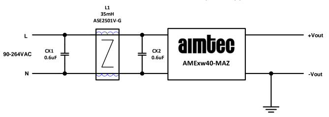
The Application circuit is EMC compliant for any type of Earth/Ground connection: Input Ground connection, Output Ground connection as shown or both sides, which is not recommended if the product Isolation is used as a Safety feature.
