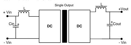
If it is required to decrease the input/output ripple, an "LC" filtering network may be connected to the input and output of the converter, see above.
