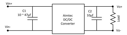
Note: Greater noise filtering can be achieved with additional capacitors, however the largest size can not exceed maximum capacitive load specification.
