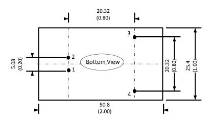
Notes: All dimensions are typical in millimeters (inches). Tolerance ±0.25 (±0.01)
