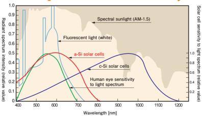
Light wavelength differs depending on the light sources to which they are exposed. Spectral sensitivity of solar cells also differs depending on the category.
