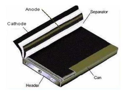
A cell is made of cathode, anode, seperator, can and header.
