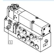
1 Electrical connection, plug 4-pin, M8, to EN 60947-5-2
