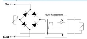
Each solenoid coil MPA is protected with a spark arresting protective circuit as well as against polarity reversal.
