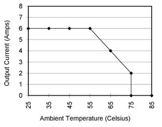
Figure 4: Derating curve
