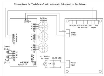
**Figure 3:** Connection diagram for interface of Tachscan-3 and Aurora.
