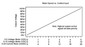
Figure 2: Motor voltage vs. analog control signal input
