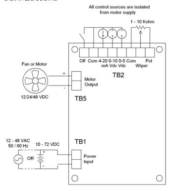
Figure 1: Aurora connections diagram
