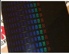
The Celsi-Reverso® (CR) are custom designed, flexible, reversible LC (liquid crystal) thermometer strips. Available ranges between -35°C to +90°C. These LC strips do change colour according to the temperature level exposed. Number turning green shows the actual temperature level.
