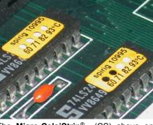
The Micro-CelsiStrip® (CS) above on the right hand IC pack has the originally white temperature sensible spots 60°C and 71 °C permanently (irreversible) blackened, a clear proof that these two temperature levels had been exceeded in the past. The still white 82°C and 93°C there have not been reaching their specific colour change levels.
