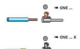
CNE ... X : for conductors with bush terminal
