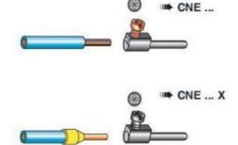
CNE ... X : for conductors with bush terminal - inserts without plate for section conductors: 0.25 - 2.5 mm2 - AWG 24 - 14
