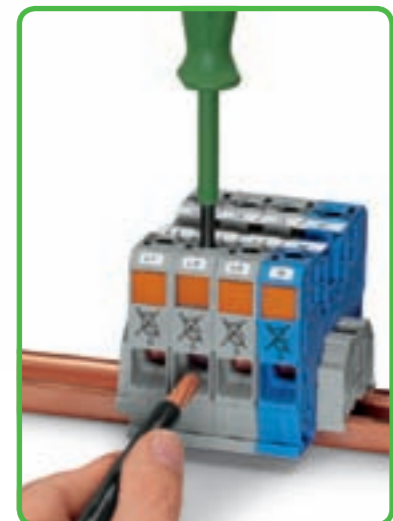
Introduce stripped wire into the clamping unit up to the stop and hold it in position . . .
