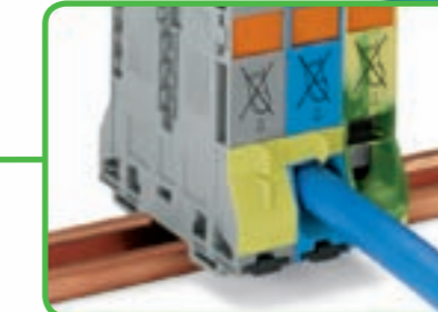
Covers provide touchproof safety by closing unused clamping units and jumper contact slots (detach the cover of the jumper contact slot from the touch protection cover of the clamping unit)
