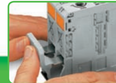
Commoning with adjacent jumper. Insertion of jumper above the conductor entry hole, without tools. Rated cross section is still 50 mm 2 /AWG 2/0 and 95 mm 2 /AWG 4/0.
