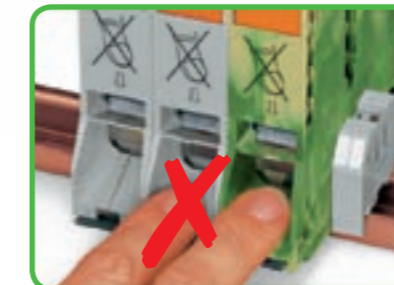
Attention! Health hazard! Keep your fingers out of the conductor entry hole!
