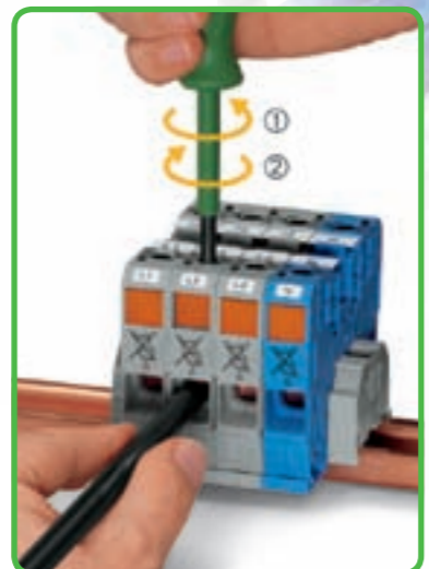
. . . A small counter-clockwise rotation releases the latch ①. Once the screwdriver ② has been removed the conductor is clamped safely.
