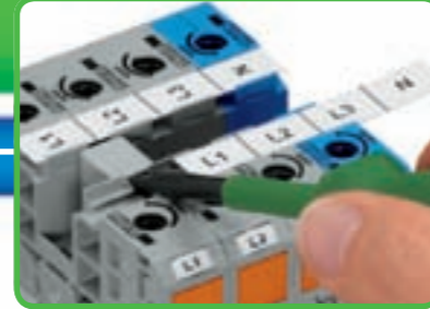
Move the marking strip laterally to remove the jumper.
