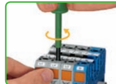
Counter-clockwise rotation using a screwdriver (blade width 5.5 mm). Hold clamp in open position using the latch.
