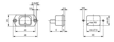
E: Solder terminals 20.5 mm E: Quick connect terminals 23.5 mm
