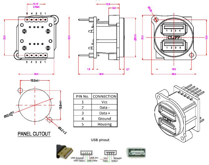
USB is a serial bus. It uses 4 shielded wires: two for power (+5v & GND) and two for differential data signals (labelled as D+ and D- in pinout)
