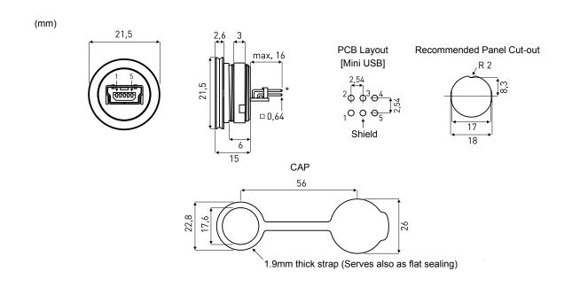
M16-Panel mount connector Frontmounting, Mini USB 2.0 Type AB
