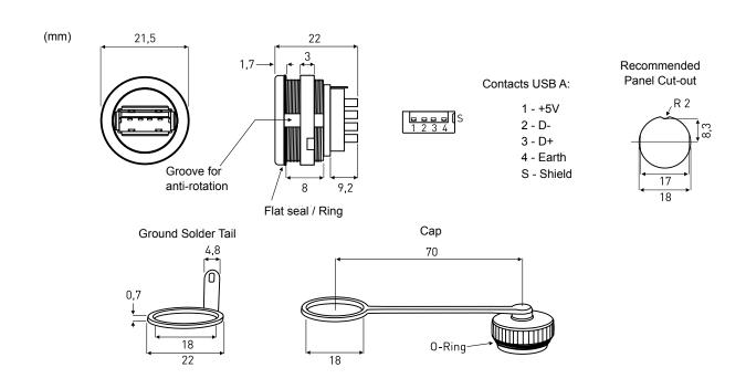
M16-Panel mount connector + Ground Solder Tail Frontmounting, USB 2.0 Type A
