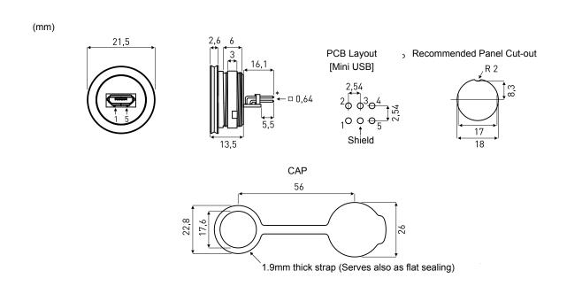
M16-Panel mount connector Frontmounting, Micro USB 2.0 Type B
